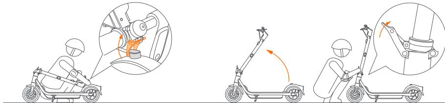
1 EN Disengage the snap hook from the buckle.
