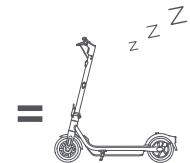
EN When the scooter is not powered on for about 7 consecutive days and its battery level is less than 30%, the battery will enter into sleep mode. If this happens, your scooter cannot be powered on. Please charge the scooter.
