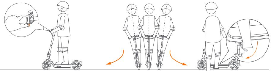
**5** EN Toggle the direction indicator button to the left/right when turning left/right.
