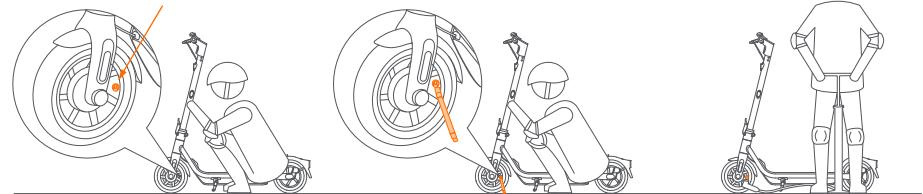
1 EN Unscrew the valve cap.
