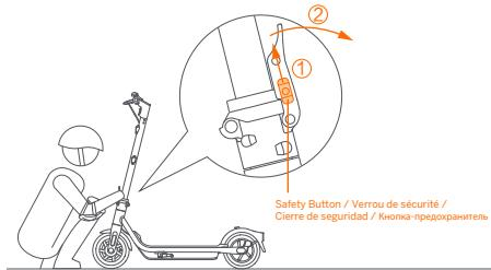
1 EN Lift the safety button and open the quick-release lever.
