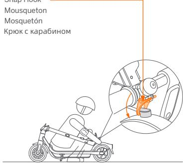
3 EN Align and fasten the snap hook to the buckle.
