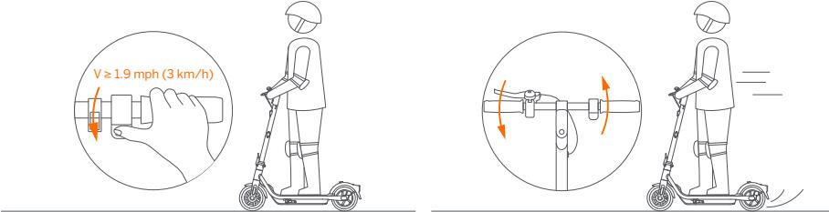
3 EN Put both feet on the footboard and stand stably. Press the throttle to speed up when you are balanced.
